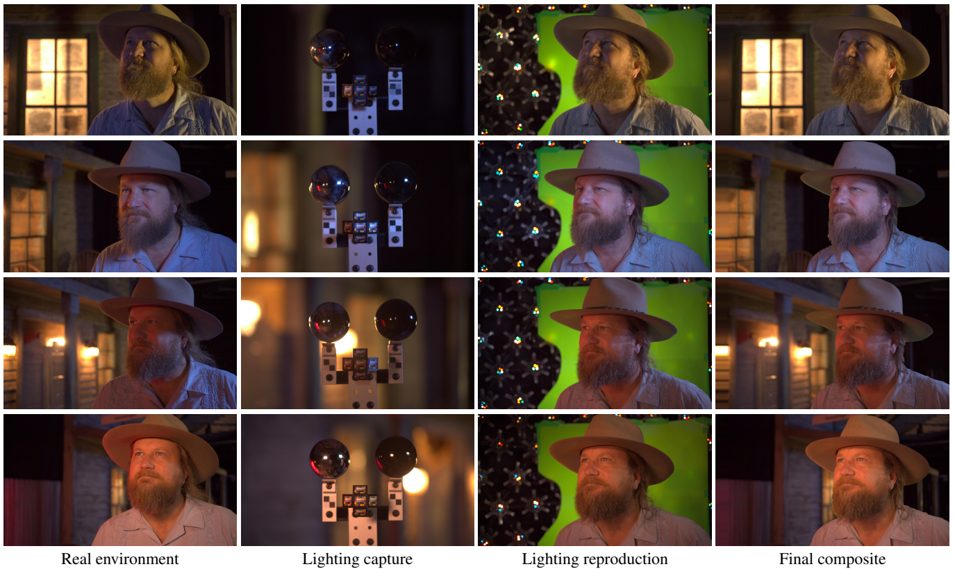
Figure 15: Frames from an image sequence where a subject moves through an environment, causing dynamic lighting from fluorescent, incandescent, and LED lights with various gels and diffusers. The last column composites the subject onto a clean plate of the set.
