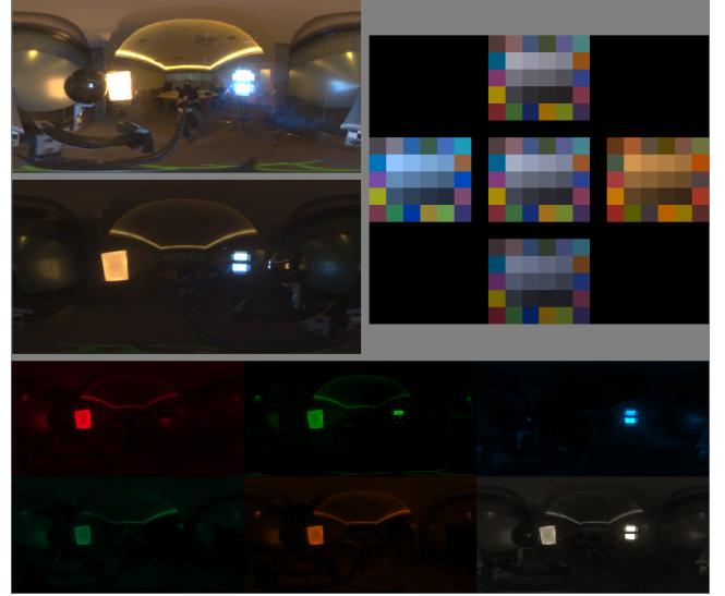
Figure 11: (upper left) Unwrapped chrome and black acrylic sphere images from Fig. 10 in latitude-longitude mapping. (upper right) Sampled colors from the five color charts. (bottom) Derived high-resolution maps for driving the red, green, blue, cyan, amber, and white LEDs to match the multispectral illumination.
