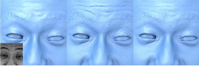
**Figure 6:** (a) Dense base mesh; (b) Proposed detail enhancement; (c) “Dark is deep” detail enhancement.
