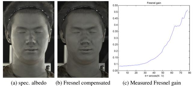
Figure 6: Data-driven Fresnel compensation from specular albedo. (a) Captured specular albedo map. (b) Specular albedo map after factoring out the measured Fresnel gain. (c) The measured view-dependent Fresnel gain (as a function of  $N \cdot V$ ) in specular albedo map used for Fresnel compensation.
