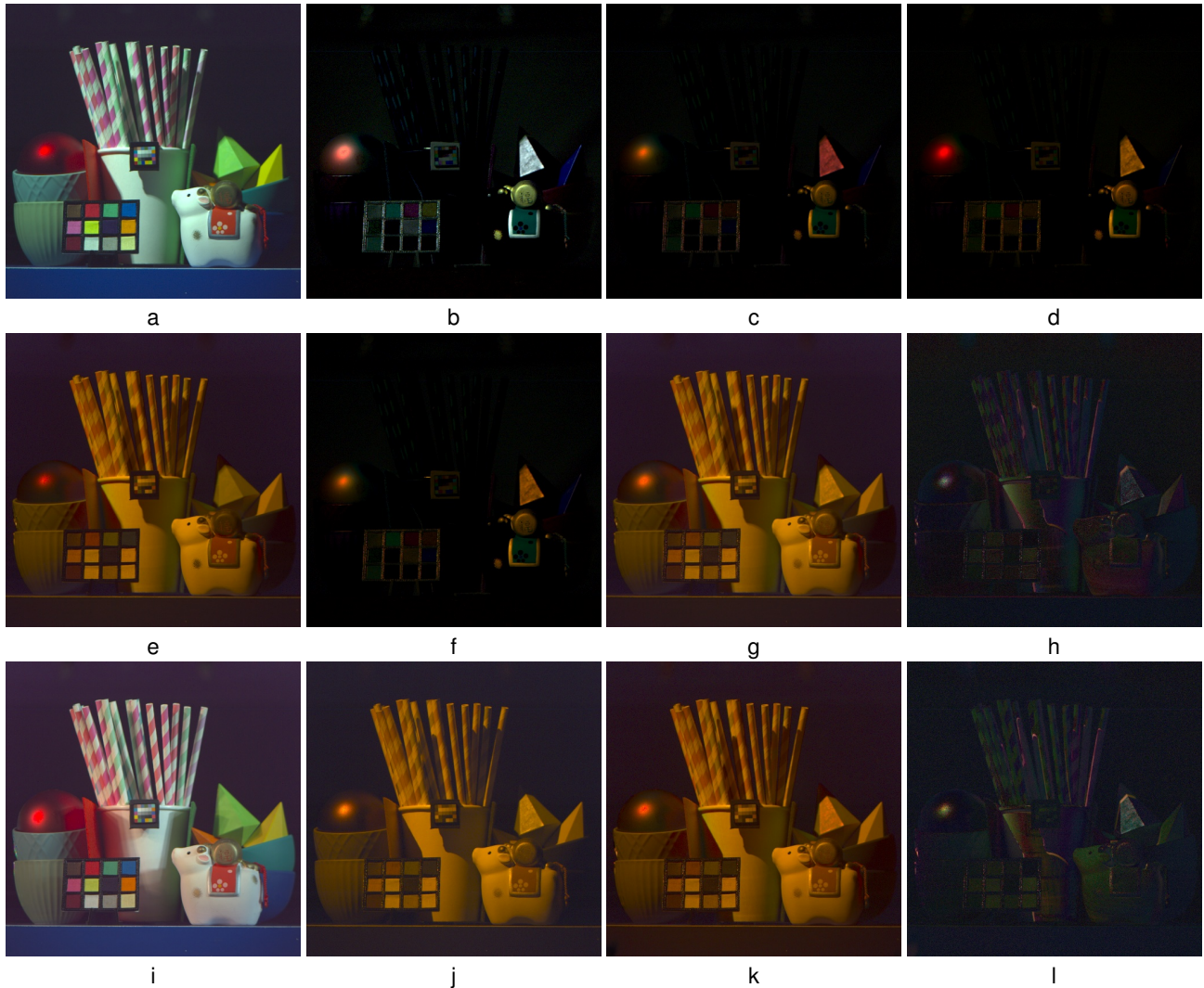
Figure 12. a. The diffuse component of the reflection of the scene. b. The specular reflection of the scene as computed from polarization difference imaging using white LEDs. c. The result of spectrally promoting the specular reflection component using Eq. 1, hallucinating the appearance under the amber LED. d. The result of spectrally promoting the specular reflection component using Eq. 3. e. The result of spectrally promoting the diffuse reflection component using Eq. 1. f. The blended result, interpolating between the images of c and d according to our approach. g. The sum of the spectrally-promoted diffuse reflection component and the blended result spectrally-promoted specular component. h. The absolute difference between g and the real lighting basis image j . i. The multispectral IBRL result using polarizing difference imaging, with the multispectral reflectance field computed in the same manner as g . j. The actual appearance of the scene when lit by the amber LED for this direction of the LED dome. k. The result of promoting both the diffuse and specular components of the reflection of the scene using 1, equivalent to the sum of e and c . l. The absolute difference between k and the real lighting basis image j .
