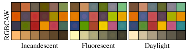
Figure 6: Charts photographed with a Canon 1DX camera (background squares) with lighting reproduced in the LED sphere photographed by a Nikon D90 camera (foreground circles).
