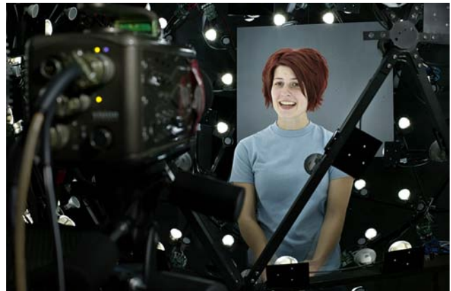
Figure 2: The lighting apparatus used for capturing a performance under time-multiplexed illumination. Behind the actor is the gray background matte surface, and at left is the high-speed camera.
