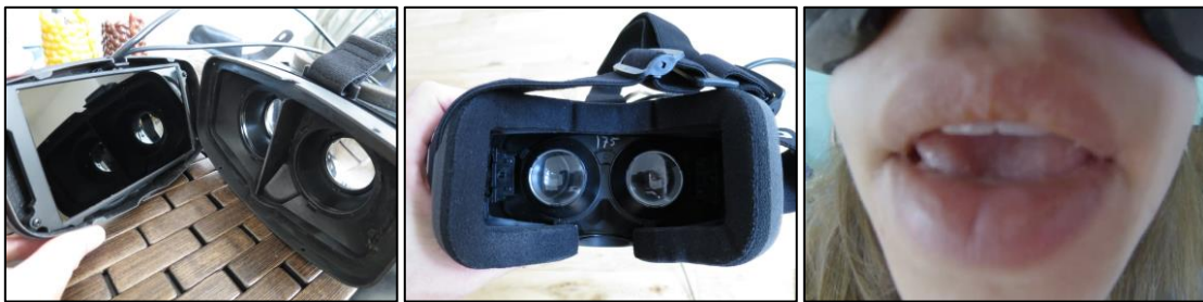
Fig. 1. (Left) An HD Oculus Rift HMD taken apart to show the 6" flat-panel display and lens optics. (Center) The facial interface of the Oculus rift, showing where motion sensors may be placed. (Right) View of an HMD wearer's mouth while speaking from a camera attached below the back edge of the HMD.
