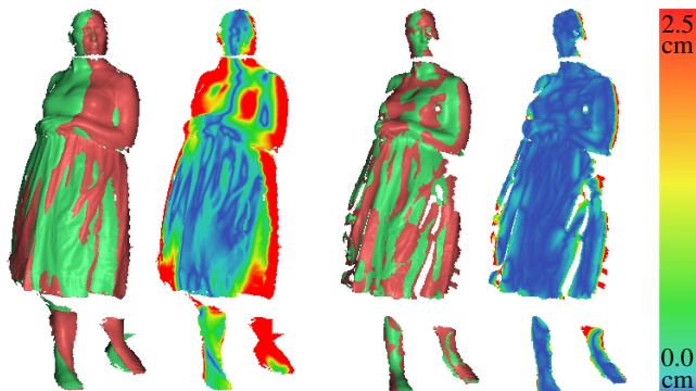
Figure 7: The integrated surfaces before matching (left) are far from each other, while the deformed surfaces after matching (right) are much closer to each other. Within each pair, the leftmost visualization shows the two meshes (in different colors) overlaid on each other, while the rightmost visualization is a color-coding of mesh-to-mesh distance.
