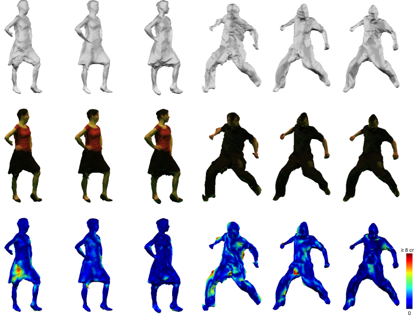
Fig. 5: Reconstructions with different views. Top to bottom rows: reconstructed mesh, textured mesh, and error visualization. Left to right columns: three-view results, four-view results, and eight-view-view results, for both two test cases respectively. Median mesh-to-scan distance: left subject: 0.84cm (three-view), 0.77cm (four-view), 0.45cm (eight-view); right subject: 1.38cm (three-view), 1.06cm (four-view), 0.59cm (eight-view).
