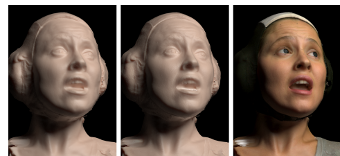
Figure 6: Subsets of the captured information. Left to right: Raw geometry, addition of normal map, addition of diffuse and specular albedo maps.
