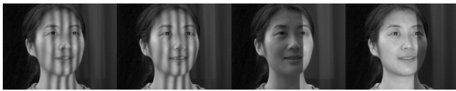
Figure 3: Patterns used for 3D face scanning, including two phase-shifted sinusoids and two half-lit images. The set of patterns is repeated at 30Hz.
