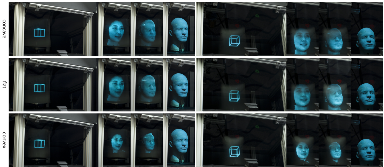
Figure 10: Comparison of the different mirror shapes for simultaneously tracked upper and lower views. (Row 1) Concave mirror (Row 2) Flat mirror (Row 3) Convex mirror. For the convex mirror, the geometry was scaled by 0.75 to fit within the smaller display volume. In the 4th and 6th columns we replaced the mirror with the actual mannequin head to provide a ground truth reference.
