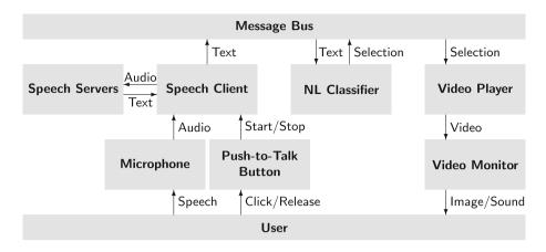
Fig. 3. System architecture
