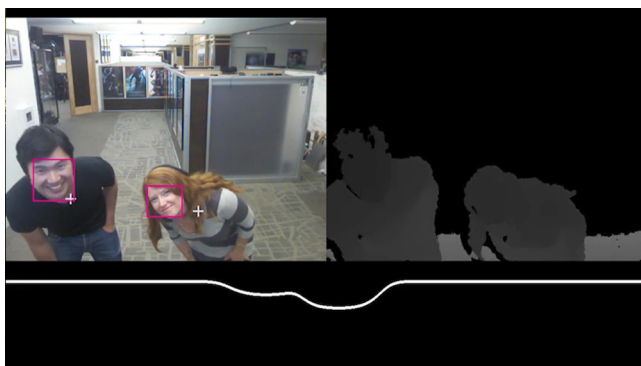
Video 3 Two viewers are tracked by the Microsoft Kinect depth camera. The graph shows the continuous estimate of viewer height that is interpolated using a smooth Gaussian falloff function (MOV, 16.3 MB) [URI: http://dx.doi.org/10.1117/1.JEI.23.1.011005.3 ].
