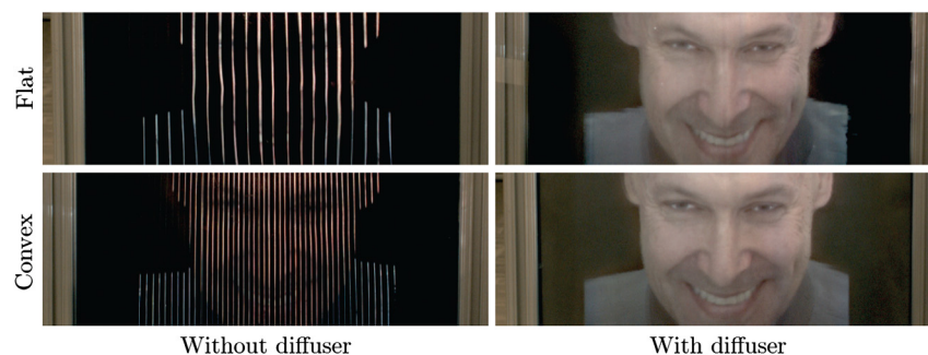
Fig. 2 The anisotropic screen forms a series of vertical lines, each corresponding to a projector lens. A 1- to 2-deg horizontal diffuser is used to blend the lines and create a continuous image. The top rows show stripes and imagery reflected on a flat anisotropic screen. The bottom row shows imagery reflected on a convex anisotropic screen. By varying the curvature of a mirrored anisotropic screen, we can decrease the pitch between reflected projector stripes. This increases the spatial resolution at the screen depth at the expense of overall angular resolution and depth of field.
