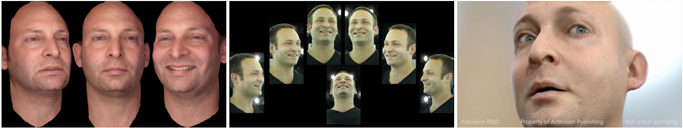
Figure 1: (Left) Three of eight high-res (0.1mm) light stage scans of the actor in static expressions. (Middle) Seven-camera HD performance recording. (Right) 180Hz video-driven blendshape model with screen-space subsurface scattering and advanced eye shading effects.
