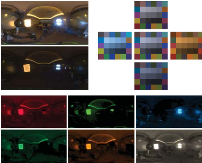
Figure 11: (upper left) Unwrapped chrome and black acrylic sphere images from Fig. 10 in latitude-longitude mapping. (upper right) Sampled colors from the five color charts. (bottom) The six derived maps for driving the red, green, blue, cyan, amber, and white LEDs to reproduce the multispectral illumination.
