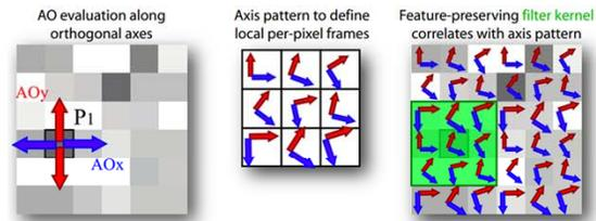
**Figure 1: Principle:** our separable approximation combines two 1D evaluations in orthogonal screen directions (e.g. x,y axis, left). By changing coordinate frames per pixel, we can derive a stochastically valid approximation of the 2D occlusion by combining the result of neighboring samples.
