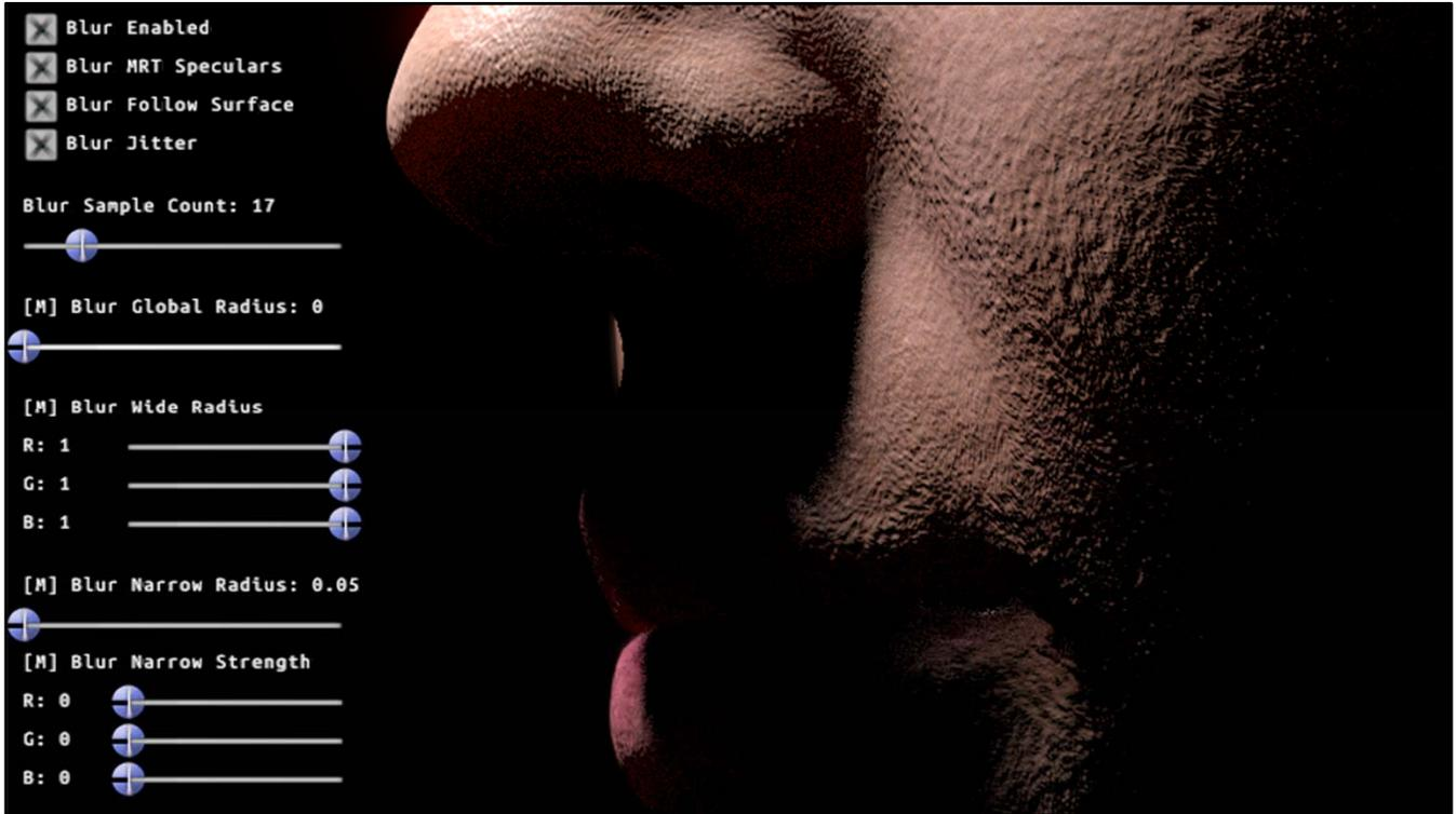
To create a subsurface scattering profile, you first adjust how far the light reaches in world space...
