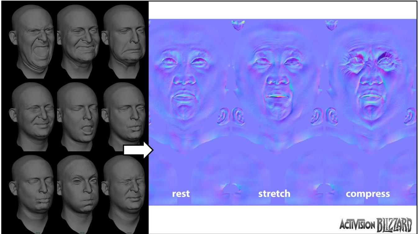
From our 30 high res meshes, We compute 3 normal maps, one at rest one at compression and one at stretch.
