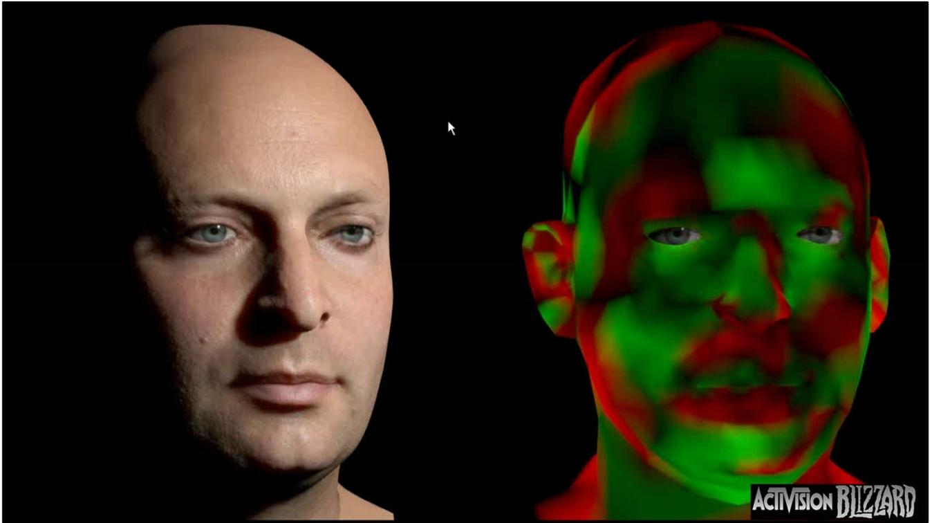
The result of blending normals, displacement and albedo maps. Driving the mesh with 70 bones, 3000 point mesh.
