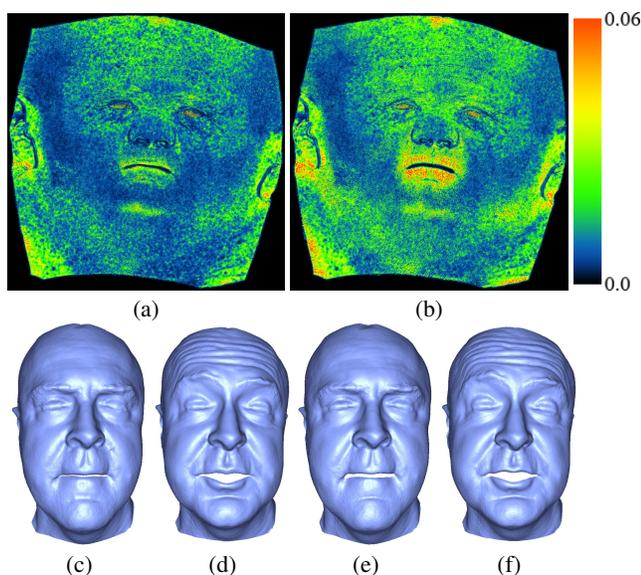
**Figure 15:** Top row: Temporal variance of contrast-normalized texture (false color, where blue is lowest and red is highest), with (a) the proposed method and (b) the method of [Beeler et al. 2011]. The variance of the proposed method is substantially lower, indicating a more consistent texture alignment throughout the sequence. Bottom row: Geometry for frames 120 and 330 of the sequence, with (c, d) the proposed method and (e, f) the prior work.
