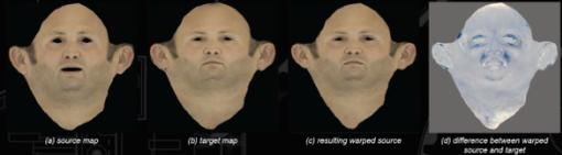
Figure 1: the original neutral expression (a) and the second expression (b) are imported into Vuvuzela. After processing, the original second expression is warped into the same texture space (c) as the neutral expression (a). The difference from the computed warp can be seen to the right (d).
