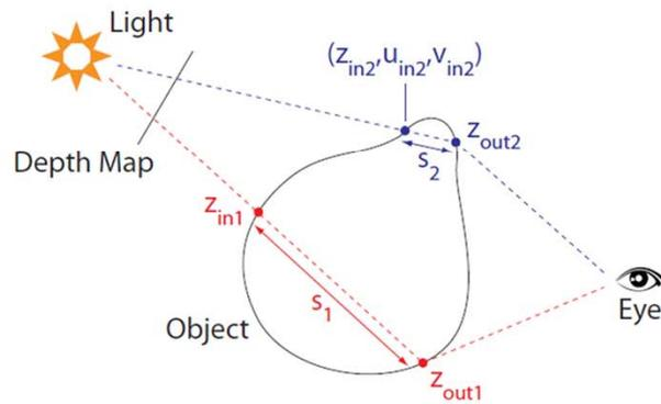
To summarize: in our previous work, we calculate the distance light travels through an object using shadow mapping, comparing current shader position  $z_{out1}$  with shadow map position  $z_{in1}$ .
