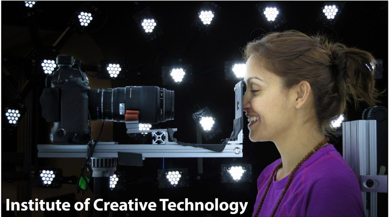
In summary: they capture micro-scale details for tiny patches of the skin – in this case the nose – and smartly clone it over the face, which allows us to accurately capture the skin reflection structure and properties.
