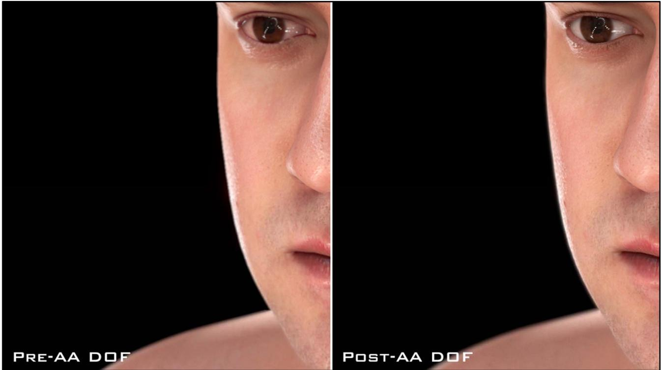
Here you can see how this pipeline order improves depth of field stability, producing more natural results under motion.
