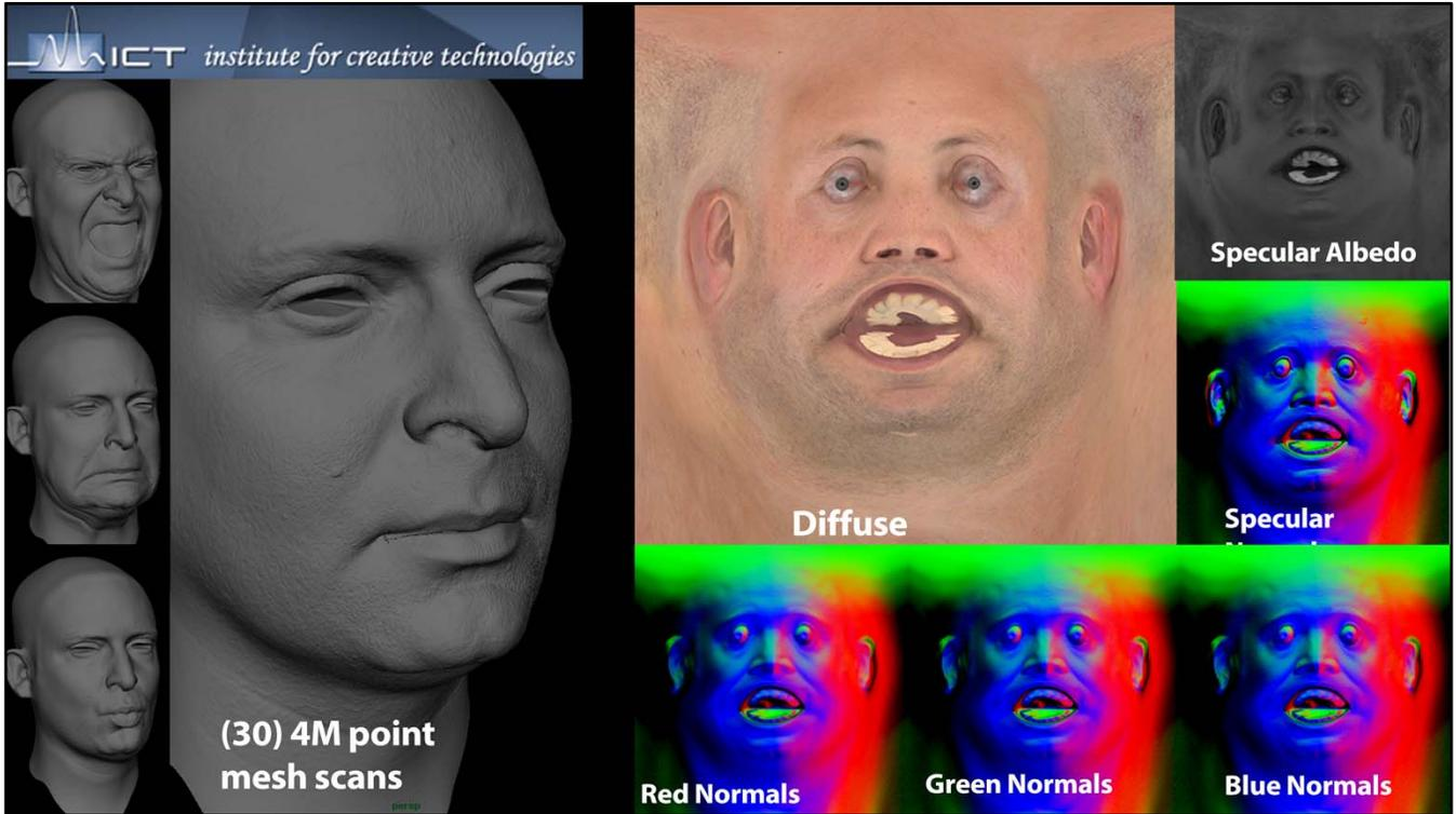
The high resolution scans were accompanied with RGB Normals, Specular normals, Specular Intensity and a Diffuse albedo. This data was captured with the Lightstage X. For this work we only utilized the high resolution scans and the diffuse albedo maps.
