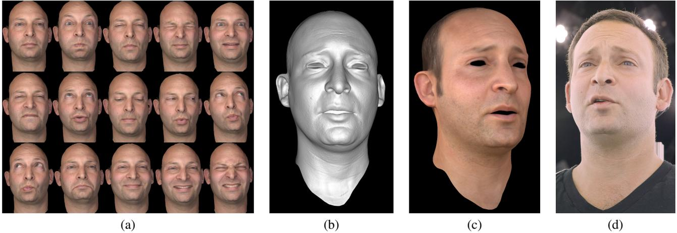
**Figure 1:** (a) High resolution geometric and reflectance information from multiple static expression scans is automatically combined with (d) dynamic video frames to recover (b) matching animated high resolution performance geometry that can be (c) relit under novel illumination from a novel viewpoint. In this example, the performance is recovered using only the single camera viewpoint in (d).
