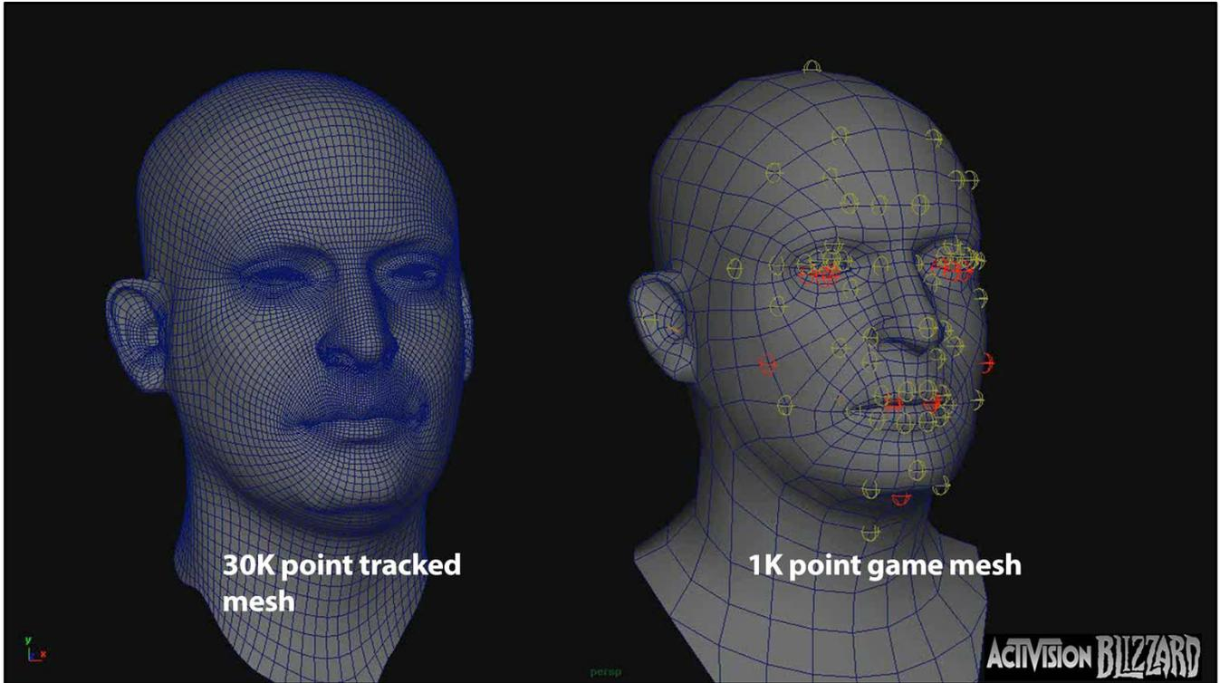
Starting with the low frequency deformation we interpret the denser deformation as a series of animated bone and bone weights.
