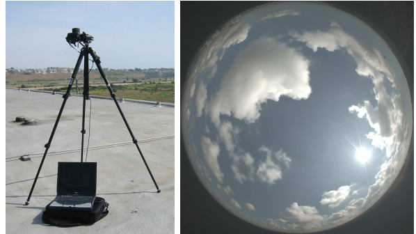
Figure 1: The camera with 180° fisheye lens and laptop on the roof of our building (left). This is a typical assembled probe (right) taken with the fish-eye lens and neutral density filter spanning the 17 stops of the sky and sun.
