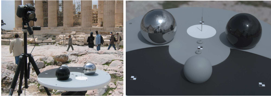
Figure 2.1: The original lighting capture board (aka. the Prober ) included a steel ball bearing, a black plastic sphere, and a spray-painted grey diffuse sphere.
