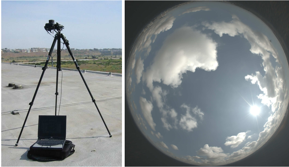
Figure 3.1: The camera with 180° fisheye lens and laptop on the roof of the USC’s Institute for Creative Technologies building (left). This is a typical assembled light probe (right) taken with the fisheye lens and neutral density filter spanning the 17 stops of the sky and sun.
