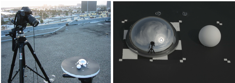
Figure 2.1: The original lighting capture board (aka. the Prober ) included a steel ball bearing, a black plastic sphere, and a spray-painted grey diffuse sphere.
